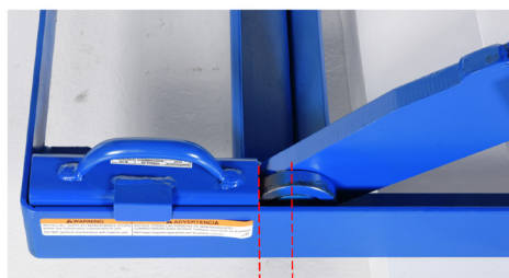
Raise the platform so that the rollers are 1"-1 1/2" away from the maintenance stops
